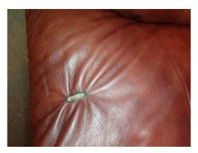
This photo represents burn damage close to the front edge of a seat cushion.
